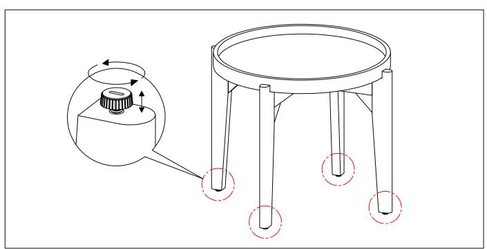
Please note stoppers on base of feet can be tightened or loosened for placement on uneven surfaces.
