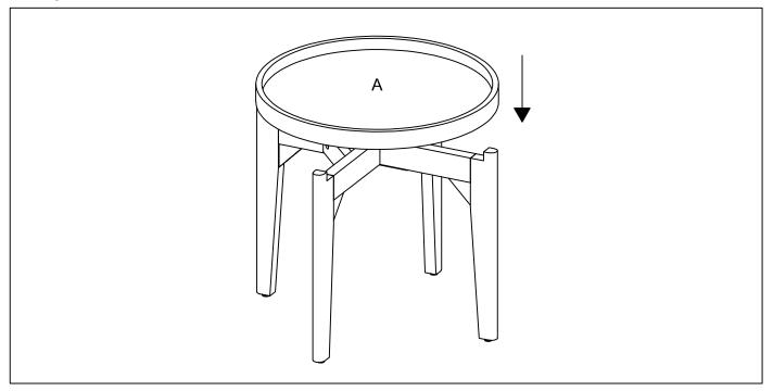
Turn leg assembly right side up, place Tray (A) inside Leg assembly.
