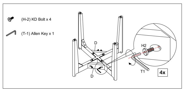
Attach Corner (D) into Leg frame shown above, then fasten all Bolts (H-2) securely using Allen Key (T-1). Tighten all the Bolts.
