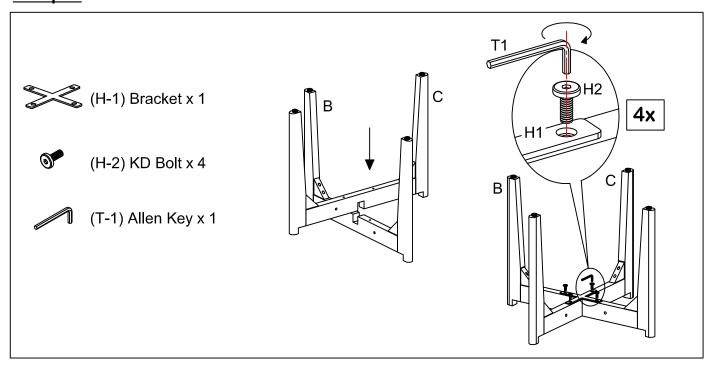
Turn Leg (B) upside down on a clean non-marring surface. Attach Leg (C) on Leg (B) shown above. Align Bracket (H-1) in center of leg assembly then fasten all Bolts (H-2) securely using Allen Key (T-1). Do not fully tighten.
